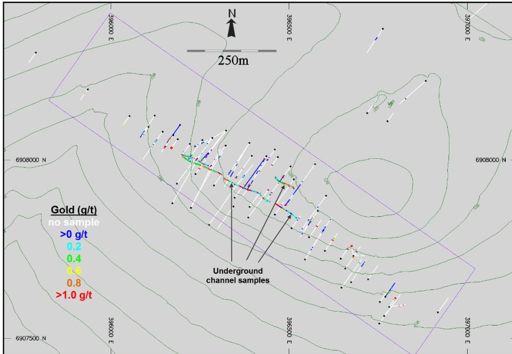
**Figure 14-50: Isometric View Looking Northwest Showing Gold Data in Drilling at Tinta Hill**
