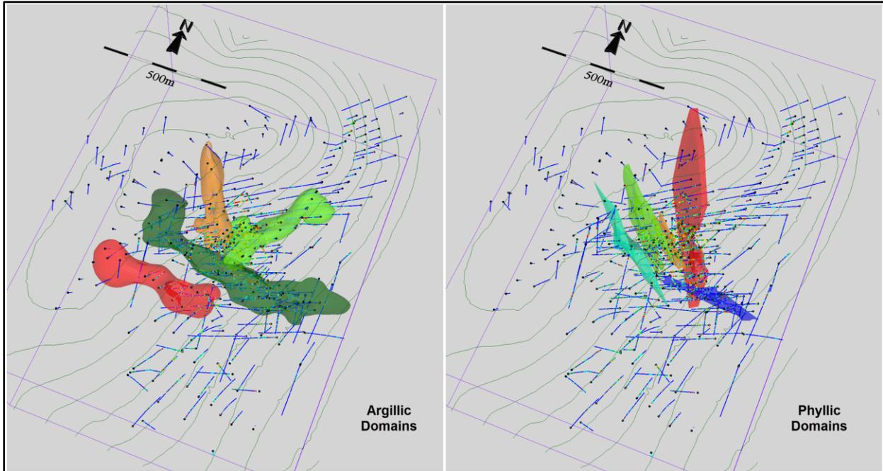
**Figure 14-9: Isometric Views Showing Faults and QFP Dykes at Nucleus**
