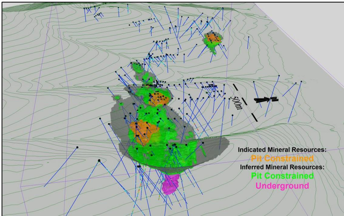
**Figure 14-63: Isometric View of Inferred Mineral Resources at the Tinta Hill Deposit**
