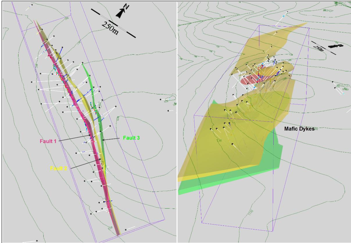
**Figure 14-52: Isometric Views of Alteration Domains at Tinta Hill**
