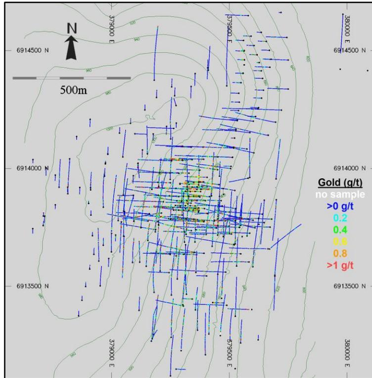
Figure 14-2: Isometric View Looking Northeast Showing Gold Data in Drilling at Nucleus
