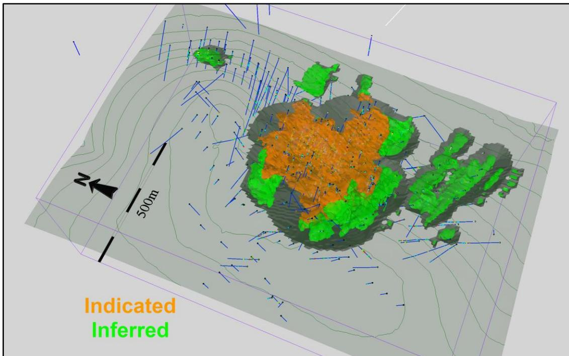
**Figure 14-61: Isometric View of Mineral Resources at the Revenue Deposit**
